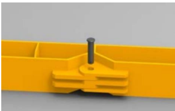
Fig. 6: pin connection of extensions
